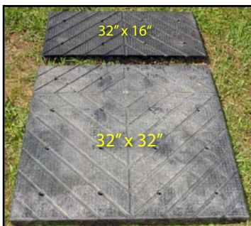
Figure 10a : This cut pattern is used in figures 5 and 6 below to supply the finishing top pieces on the sides running along the short lengths of the main panels. The cut is 16" from one end, resulting in one piece 32" x 16" and another 32" x 32".
