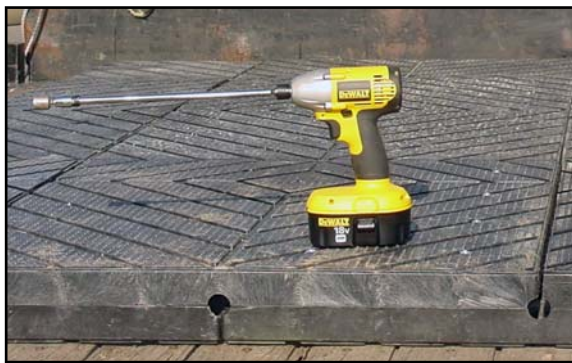
Figure 13: We highly recommend using a heavy duty cordless hammer drill and extension for tightening the bolts.
