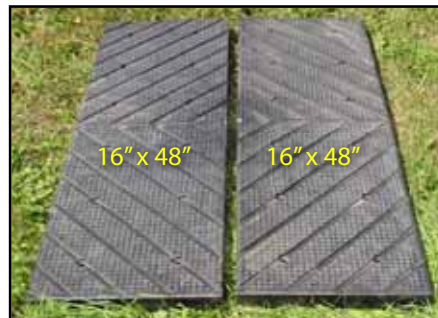
Figure 10b: This pattern is used in figures 7 and 8 below to supply the finishing top pieces on the sides running lengthways with the main panels. The panel is split lengthways down the middle leaving two equal 16" x 48" pieces.
